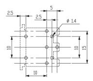
\*a distance of ground contact pins 10 mm
