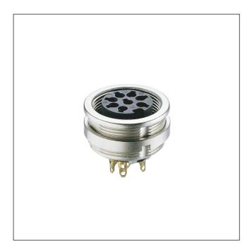
Chassis socket acc. to AISG specification and IEC 61076-2-106, IP68, with threaded joint and solder terminals, for front mounting
