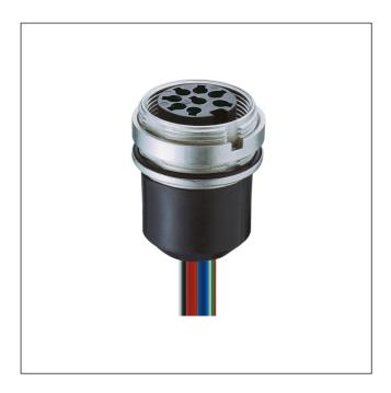
Chassis socket acc. to IEC 61076-2-106 and AISG specification, IP68, with threaded joint, cables and potted solder area, for back side mounting
