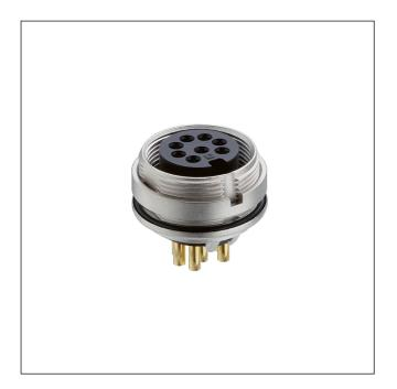
SWUM<sup>™</sup> chassis socket acc. to IEC 61076-2-106 and AISG specification, IP68/67, with threaded joint and solder terminals, for back side mounting
