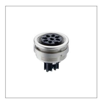
Chassis socket acc. to AISG specification and IEC 61076-2-106, IP68, with threaded joint, empty housing for reception of crimp contacts, for front mounting
