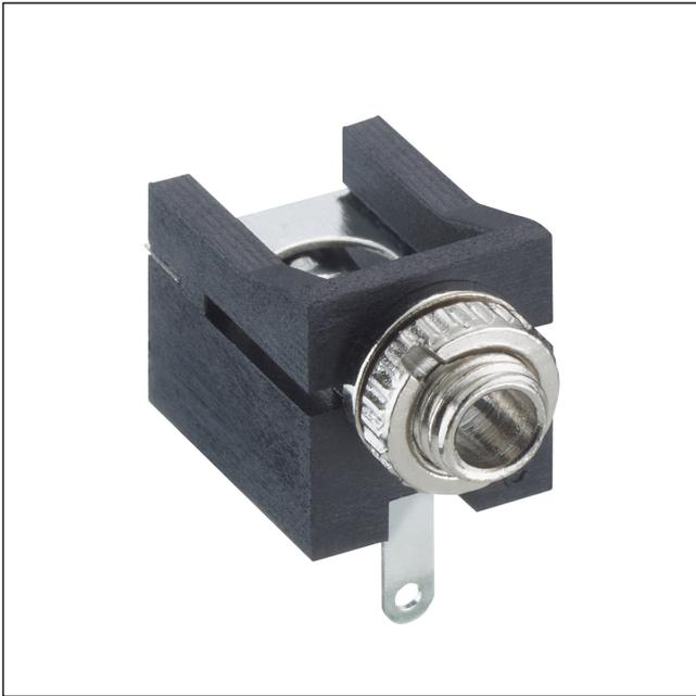
Jack chassis socket acc. to JIS C 6560 JC25P2B, 2.5 mm, 2 poles/mono, angular version, with break contact and solder eyes, for printed circuit boards, for back side mounting
