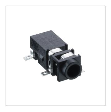
Jack chassis socket acc. to JIS C 6560 JC25J3B, 2.5 mm, 3 poles/stereo, angular version, with 2 break contacts, for printed circuit boards, surface mounting technology (SMT)
