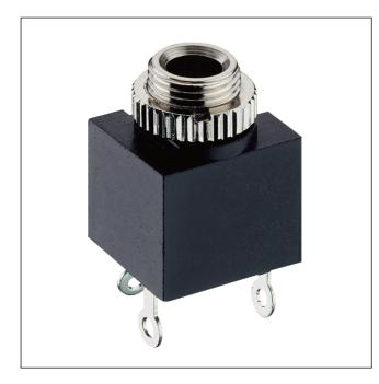
Jack chassis socket acc. to JIS C 6560 JC35J2B, 3.5 mm, 2 poles/mono, straight/upright version, with break contact and solder eyes, for printed circuit boards, for back side mounting
