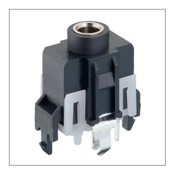
Jack chassis socket acc. to JIS C 6560 JC35J3Z, 3.5 mm, 3 poles/stereo, upright version, with break contact, for printed circuit boards, with retaining hooks
