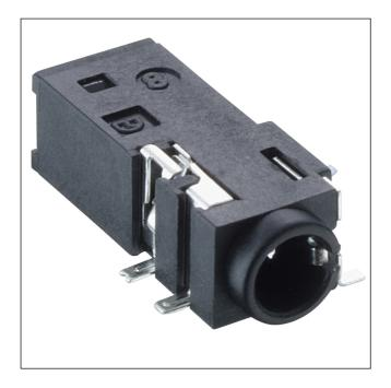
Jack chassis socket according to JEITA RC-5325A, 3.5 mm, 4 poles/stereo, with two break contacts, angular version, for printed circuit boards, surface mount technology (SMT)
