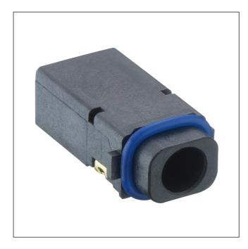
Jack chassis socket according to JEITA RC-5325A JC35J4A, 3.5 mm, 4 poles/stereo, potted and with sealing towards mounting plate, IPx7, angular version, for printed circuit boards, surface mount technology (SMT)
