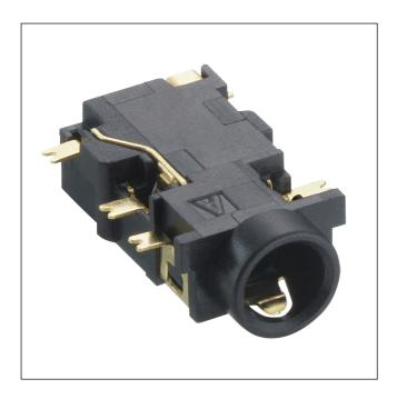
Jack chassis socket according to JEITA RC-5325A, 3.5 mm, 4 poles/stereo, with two break contacts, angular version, for printed circuit boards, surface mount technology (SMT), for mid-mount placement
