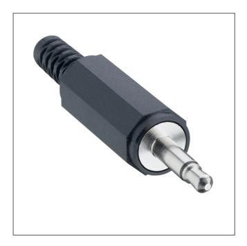
Jack plug acc. to JIS C 6560 JC35P2, 3.5 mm, 2 poles/mono, straight version, cone headed, with bend protection and solder terminals
