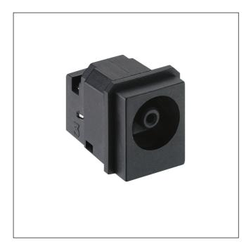
Power supply chassis socket acc. to JEITA RC-5322 JCBJ11, angular version, with break contact, for printed circuit boards
