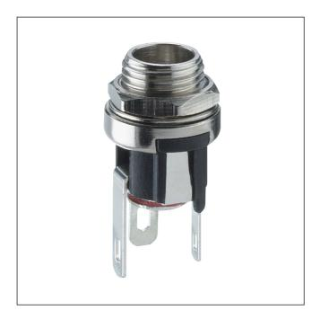
Power supply chassis socket, for plugs 5.5 mm x 2.5 mm, straight version, with break contact and solder eyes, for back side mounting
