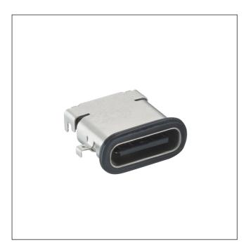
USB 3.1 chassis socket type C, 24 poles, with sealing towards mounting plate, angular version, for printed circuit boards, surface mounting technology (SMT/THR)
