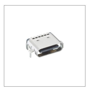
USB 3.1 chassis socket type C, 24 poles, angular version, for printed circuit boards, surface mounting technology (SMT), for mid-mount placement
