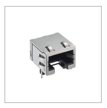
Modular chassis socket, #######, 10p10c (RJ50), angular, with full shielding, lower side locking, positioning pegs/retaining hooks and ground contacts, for printed circuit boards, surface mounting technology (SMT)
