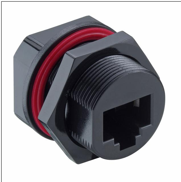
Modular chassis socket, 8p8c (RJ45), with ground contact and sealing towards mounting plate, IP68, angular version, for back side mounting, for printed circuit boards
