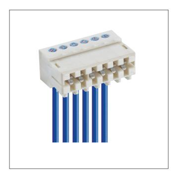
RAST 2.5 connector for direct mating, insulation displacement technology (IDT), with locking on printed circuit board by means of enhanced locking toes, alternatively with or without keying rib and closed sides, for individual conductors, daisy chain possible for printed circuit boards of 1 mm thickness contact pitch 2.5 mm
