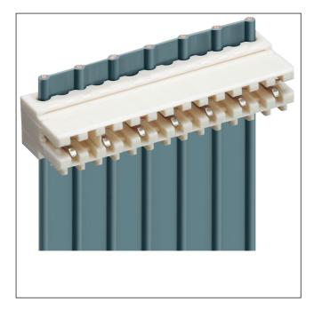
RAST 2.5 connector for direct mating, insulation displacement technology (IDT), with locking on printed circuit board by means of locking toes, alternatively with or without keying rib and closed sides, for ribbon cable, daisy chain possible, consecutive placement without loss of pitch
