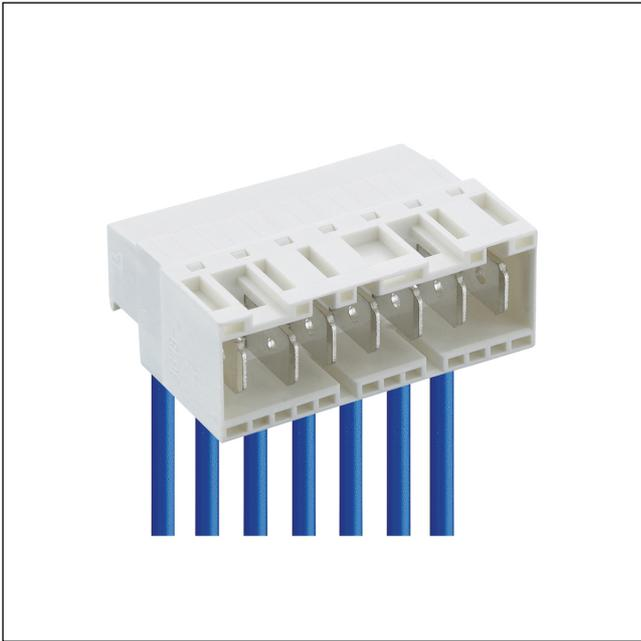
RAST 5 tab header, with screw terminal, with lift clamp with protection against misplacing, with test holes, cable departure opposite to lock, with pre-mating protective contact
