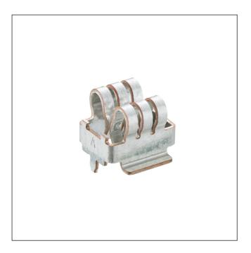
High-current contact bush with positioning pegs, in surface mount technology (SMT), mateable from top or bottom direction, for tab contacts 0.8–1.5 mm, for printed circuit boards or busbars
