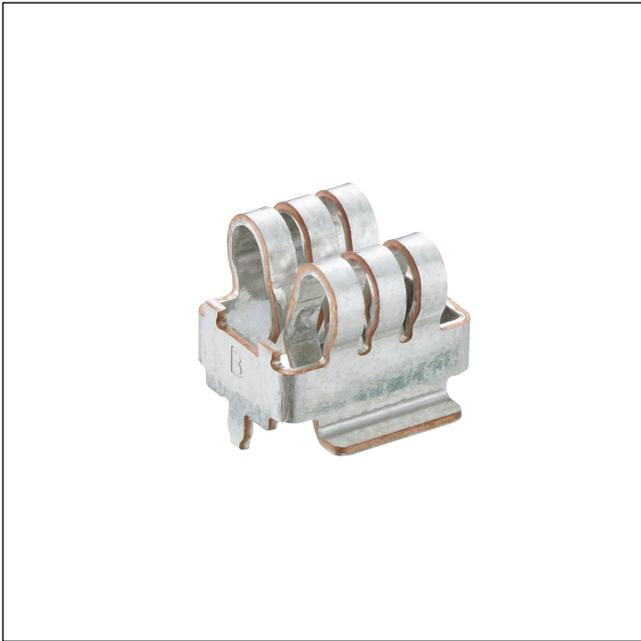
High-current contact bush with positioning pegs, in surface mount technology (SMT), mateable from top or bottom direction, for tab contacts 1.5–2.0 mm, for printed circuit boards or busbars
