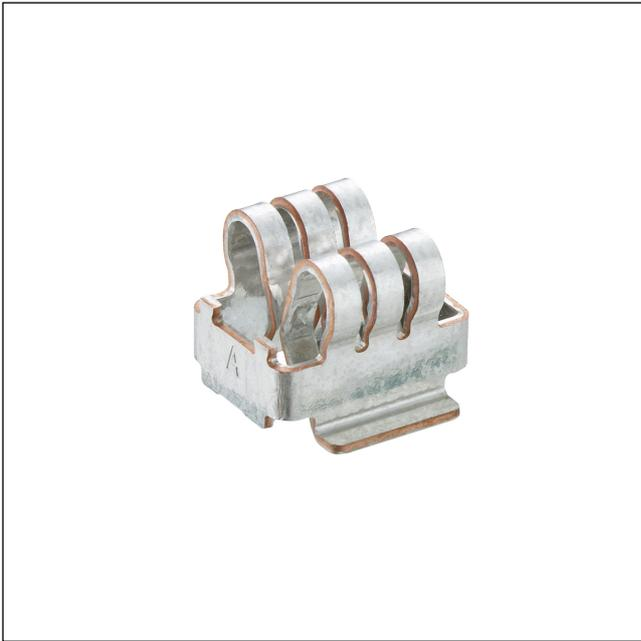
High-current contact bush, in surface mount technology (SMT), mateable from top or bottom direction, for tab contacts 0.8–1.5 mm, for printed circuit boards or busbars
