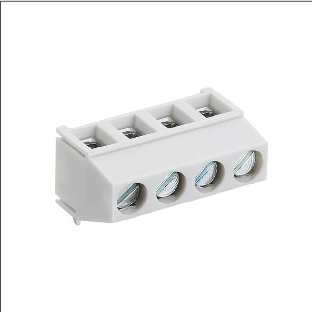
Miniature screw terminal block, with lift clamp without protection against misplacing, right angle version, with test hole, consecutive placement without loss of pitch contact pitch 5.0 mm
