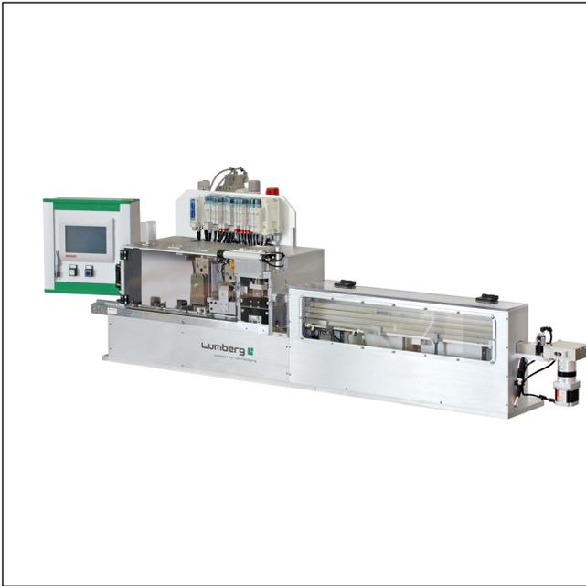
Semiautomatic harnessing machine for termination of RAST 1.5 connectors in insulation displacement technology (IDT), larger base machine, with integrated stations for cable color detection and keying cutting, individual upgrading possible
