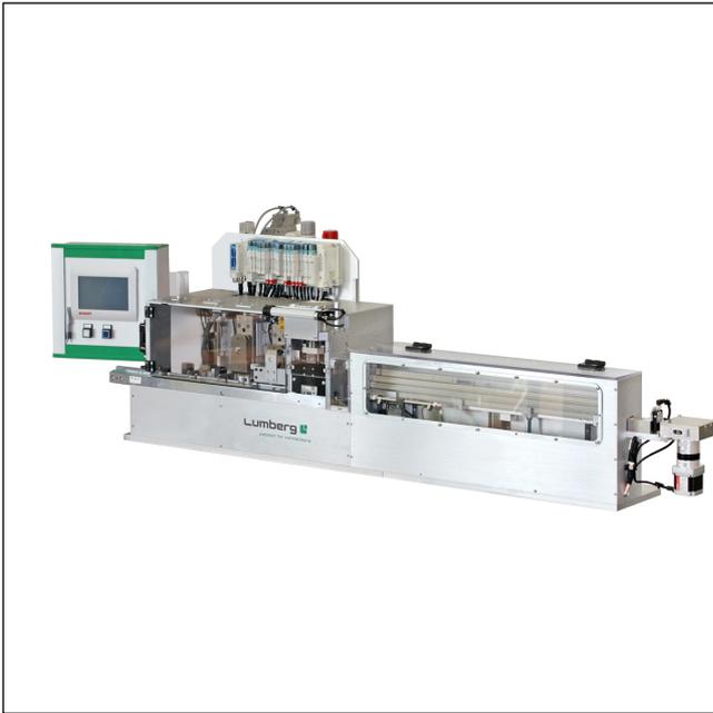
Semiautomatic harnessing machine for termination of RAST 1.5 connectors in insulation displacement technology (IDT), larger base machine, with integrated stations for cable color detection, keying cutting and keying testing, individual upgrading possible
