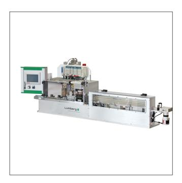
Semiautomatic harnessing machine for termination of RAST 1.5 connectors in insulation displacement technology (IDT), larger base machine, with integrated station for keying cutting, individual upgrading possible
