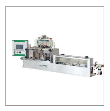
Semiautomatic harnessing machine for termination of RAST 1.5 connectors in insulation displacement technology (IDT), larger base machine, with integrated stations for keying cutting and keying testing, individual upgrading possible
