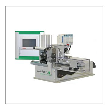
Semiautomatic harnessing machine for termination of RAST 2.5 connectors in insulation displacement technology (IDT), small base machine with integrated removal of connector chain interlinks, limited upgrading possible
