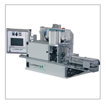
Semiautomatic harnessing machine for termination of RAST 2.5 connectors in insulation displacement technology (IDT), larger base machine, with integrated cable color detection, individual upgrading possible
