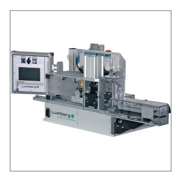
Semiautomatic harnessing machine for termination of RAST 2.5 connectors in insulation displacement technology (IDT), larger base machine, with integrated stations for cable color detection and keying cutting, individual upgrading possible
