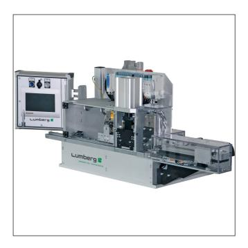
Semiautomatic harnessing machine for termination of RAST 2.5 connectors in insulation displacement technology (IDT), larger base machine, with integrated station for keying cutting, individual upgrading possible
