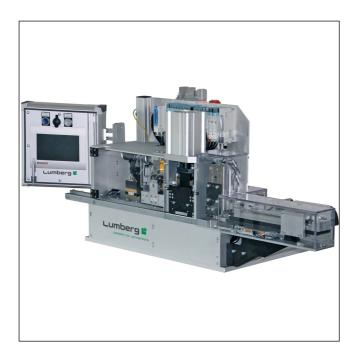
Semiautomatic harnessing machine for termination of RAST 2.5 connectors in insulation displacement technology (IDT), larger base machine, with integrated stations for keying cutting and keying testing, individual upgrading possible
