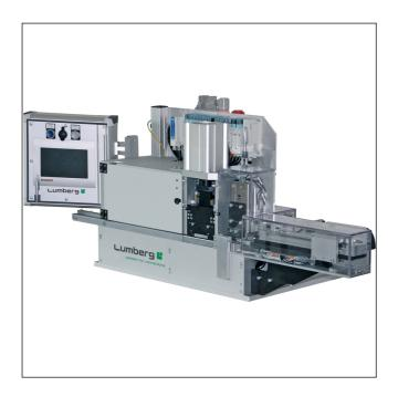
Semiautomatic harnessing machine for termination of RAST 2.5 connectors in insulation displacement technology (IDT), larger base machine, with integrated station for removal of connector chain interlinks, individual upgrading possible
