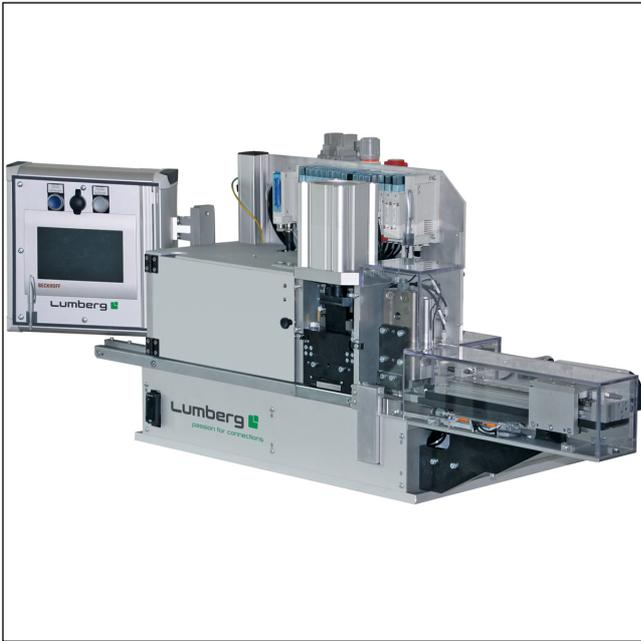
Semiautomatic harnessing machine for termination of RAST 2.5 connectors in insulation displacement technology (IDT), larger base machine, with integrated stations for removal of connector chain interlinks and cable color detection, individual upgrading possible
