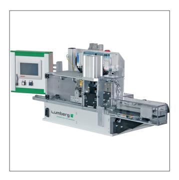
Semiautomatic harnessing machine for termination of RAST 2.5 connectors in insulation displacement technology (IDT), larger base machine, with integrated stations for removal of connector chain interlinks, cable color detection, keying cutting, individual upgrading possible
