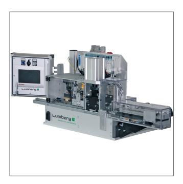
Semiautomatic harnessing machine for termination of RAST 2.5 connectors in insulation displacement technology (IDT), larger base machine, with integrated stations for removal of connector chain interlinks, cable color detection, keying cutting and keying testing, individual upgrading possible
