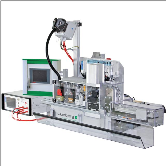
Semiautomatic harnessing machine for termination of RAST 2.5 connectors in insulation displacement technology (IDT), larger base machine, fully equipped with integrated stations for removal of connector chain interlinks, cable color detection, keying cutting, keying testing and high-voltage test
