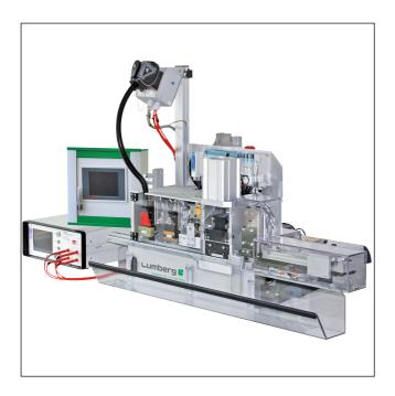
Semiautomatic harnessing machine for termination of RAST 2.5 connectors in insulation displacement technology (IDT), larger base machine, fully eqipped with integrated stations for removal of connector chain interlinks, cable color detection, keying cutting, keying testing and high-voltage test
