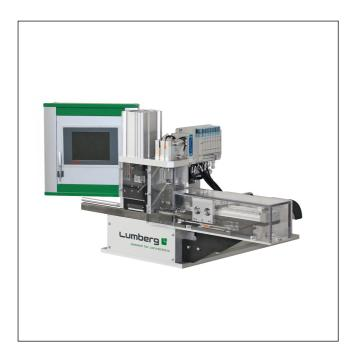
Semiautomatic harnessing machine for termination of RAST 2.5 plus™ connectors in insulation displacement technology (IDT), with integrated cable color detection
