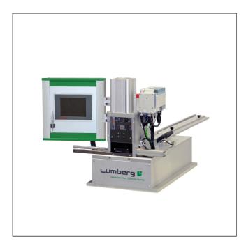
Semiautomatic harnessing machine for termination of RAST 5 connectors in insulation displacement technology (IDT)
