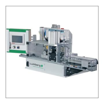
Semiautomatic harnessing machine for termination of RAST 5 connectors in insulation displacement technology (IDT), larger base machine, with integrated stations for cable color detection and keying cutting, individual upgrading possible
