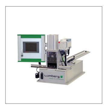
Semiautomatic harnessing machine for termination of RAST 7.5 Power connectors in insulation displacement technology (IDT), with integrated cable color detection
