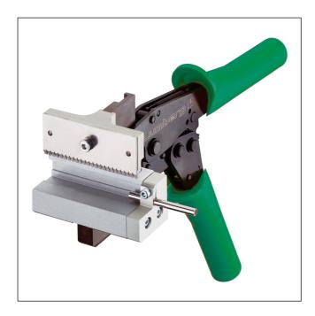
Hand tongs for keying of **pre-terminated** RAST 2.5 connectors according to RAST 2.5 standard
