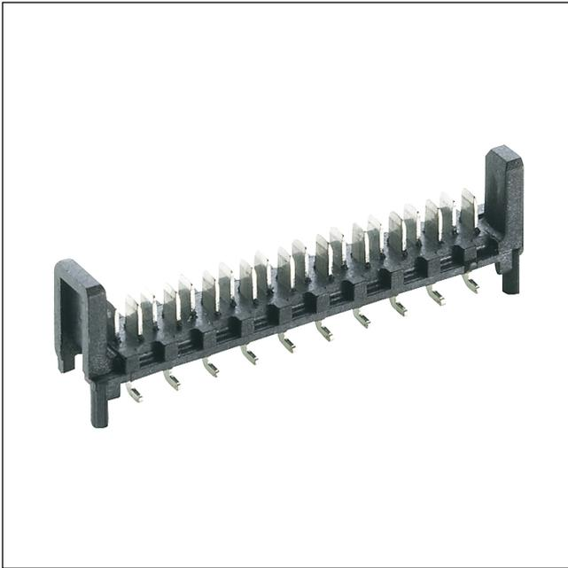
Micromodul™ tab header, upright, in surface mount technology (SMT), solder contacts dual row staggered, with press-fit spigots, in bulk, with retaining hooks
