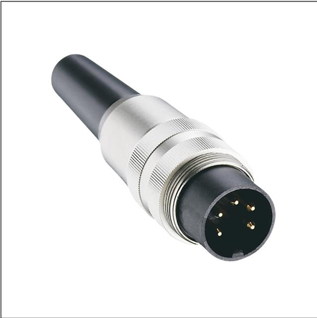
Plug acc. to IEC 61076-2-106, IP40, straight version, with threaded joint, solder terminals and bend protection, for cable diameter up to 6 mm
