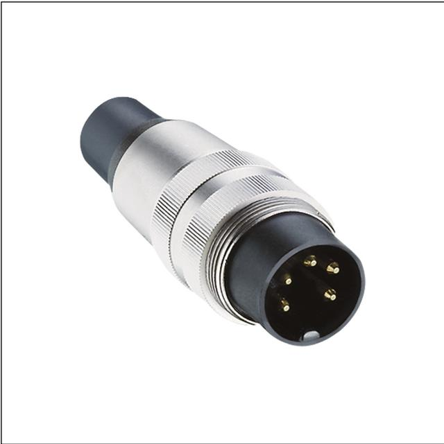
Plug acc. to IEC 61076-2-106, IP40, straight version, with threaded joint, solder terminals and bend protection, for cable diameter up to 8 mm
