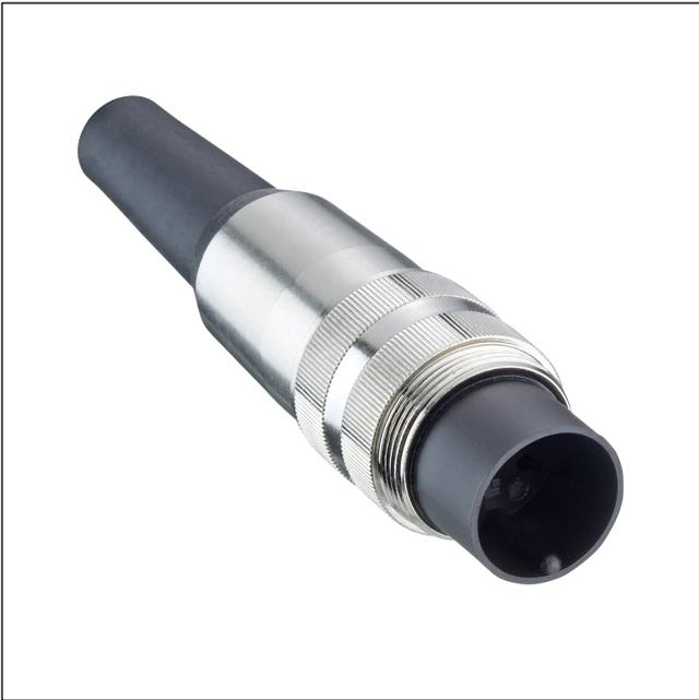
Plug acc. to IEC 61076-2-106, IP40, straight version, with threaded joint, empty housing for reception of crimp contacts, with bend protection, for cable diameter up to 6 mm
