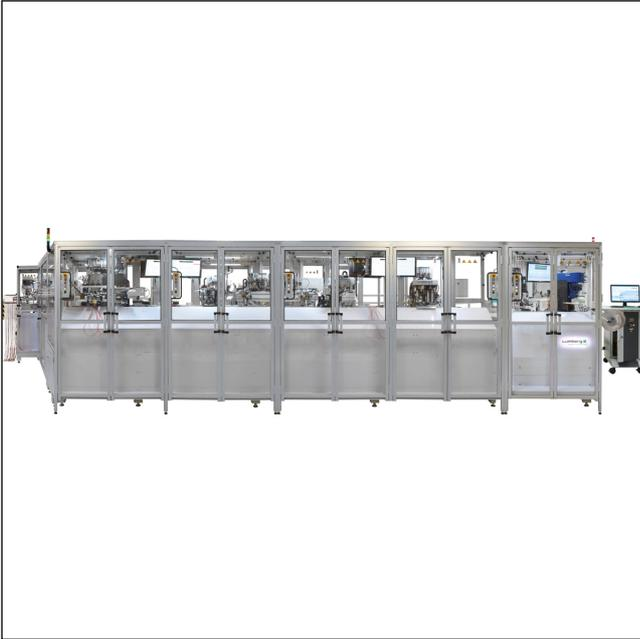
Versatile, fully automatic harnessing machine for termination of RAST connectors in insulation displacement technology (IDT), for production of daisy chain harnesses combined with additional crimp contacts, for flexible harness configurations, machine to be adapted to the application's requirements
